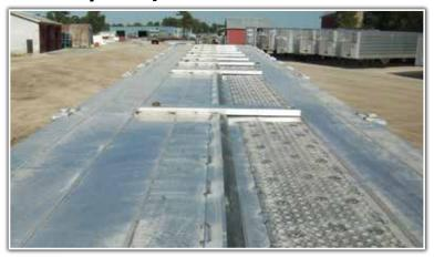
With this flip roof the trailer can be compact or top loaded. This allows the trailer to backhaul, and carry materials other than waste.
