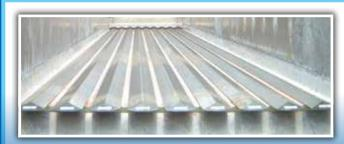
Steel V-9 Floor with 24" Steel Rear Slat Wear Strips
