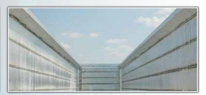
• Extreme duty tapered top rails provide structure to minimize the number of top crossmembers required in the trailer.
