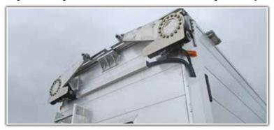
Mesh split flip roofs are hydraulically operated using front mount slew drive gear boxes. The mesh is a light weight roof option for containing the load.
