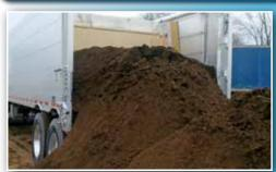
Walking floor trailer specifically designed for hauling various aggregate materials.
