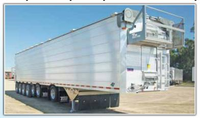
The compactor flip roofs are hydraulically operated using front mount slew drive gear boxes. Roofs are hinged at the sidewall using greasable heavy duty hinges. This allows the trailer to operate as an open or closed top trailer, providing versatility.
