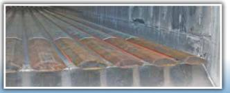
Aluminum Flat Top V-9 Floor with 48" Steel Rear Slat Extension
