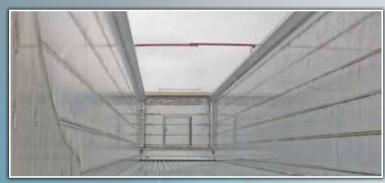
Open top trailers are designed with extruded tapered top rails to minimize build up of material during loading.
