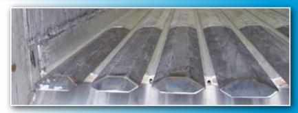
Leak Resistant floor compatible with all Keith® V-9 Walking Floor.
