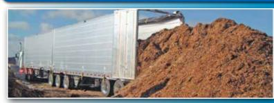
B-Train configuration, lead and pup slides together to allow material to walk from lead thru pup. Can be used on tipping platform as well.
