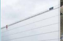
Top Rail Overlay for Top Loading Customized Tool Compartment on Loading Side of Trailer
