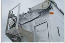
The Versitex split flip roofs are hydraulically operated using front mount slew drive gear boxes. Roofs are hinged at the sidewall using greasable heavy duty hinges. This is an excellent alternative to tarps & mesh roofs for open top trailers in terms of durability. They are comprised of a lightweight aluminum frame and Versitex composite sheet.
