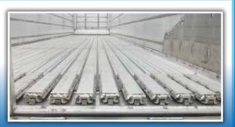
Aluminum V-18 Floor with 24" Rear Slat Wear Strips
