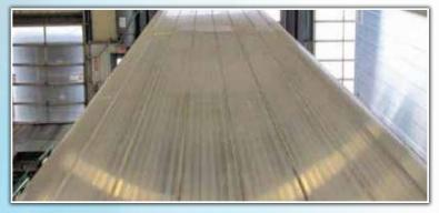
Closed top trailers feature a two-section roof. Front half consists of a lighter extruded panel profile. The rear half consists of a heavier extruded panel profile.
